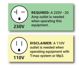
Note: Equipment comes standard in three phase configuration. Buck boosters must be installed by licensed electrician in your state/county
