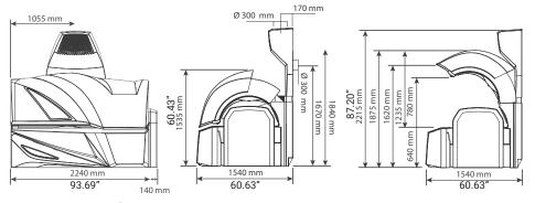
Note: Equipment comes standard in three phase configuration. Buck boosters must be installed by licensed electrician in your state/county
